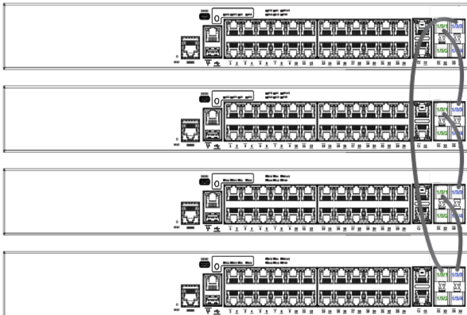
FIGURE 11 ICX 7150 24-port stack ring topology
