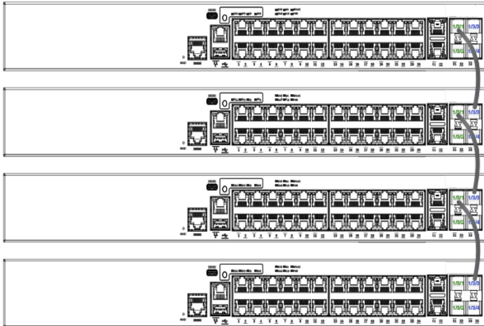
FIGURE 11 ICX 7150 24-port stack ring topology
