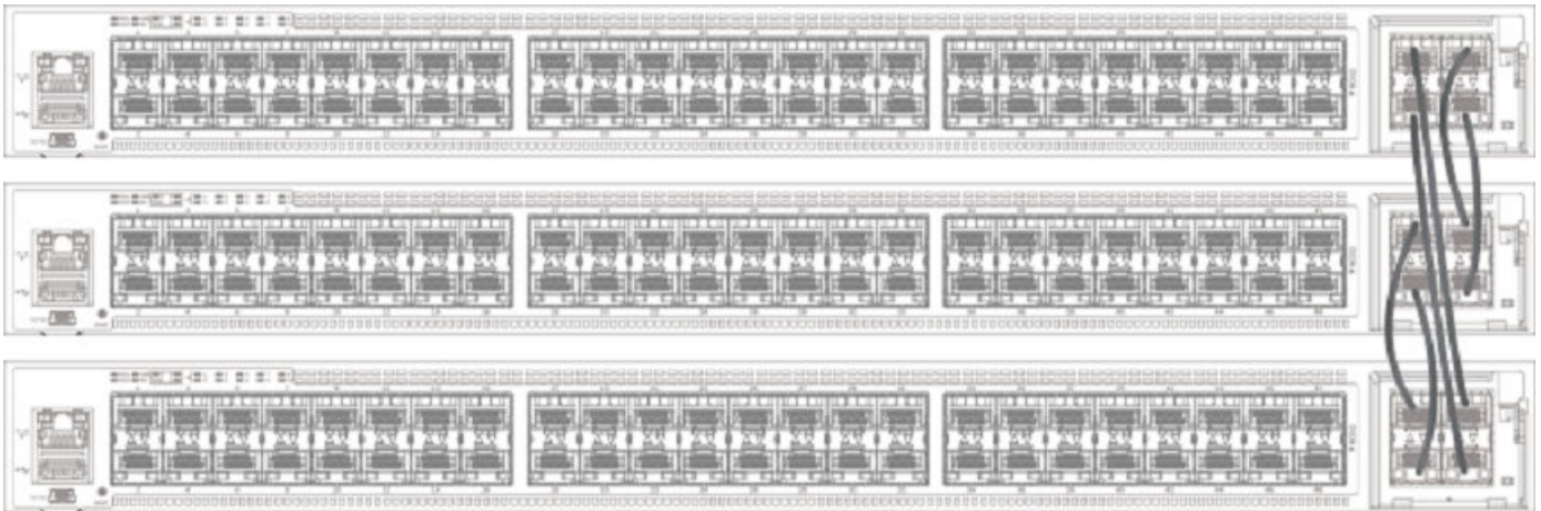
FIGURE 23 ICX 7450 4 X 10-Gbps ring using stacking trunks
