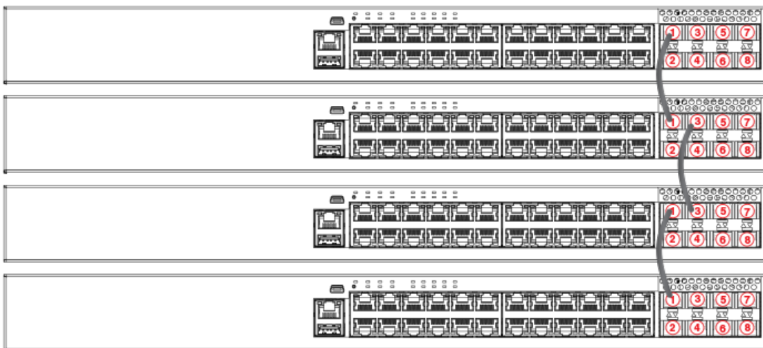
FIGURE 16 ICX 7250-24P linear stack
