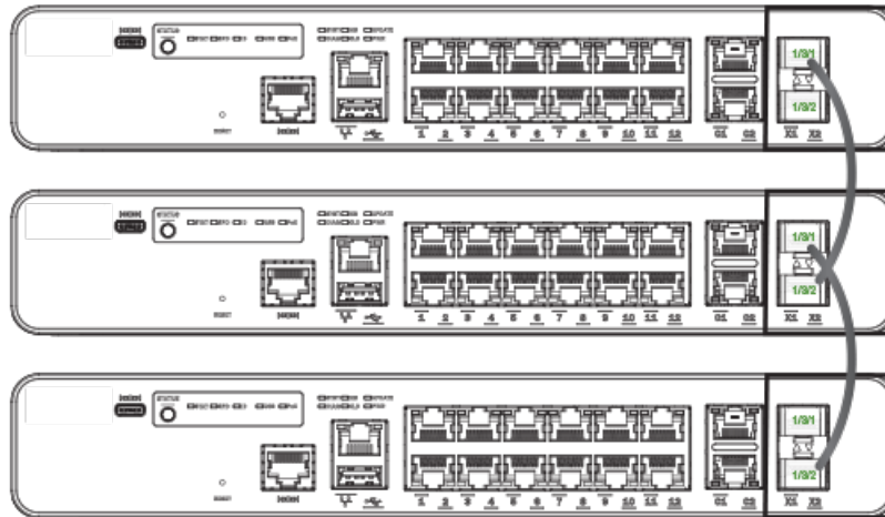
FIGURE 9 ICX 7150-C12P stack ring topology
